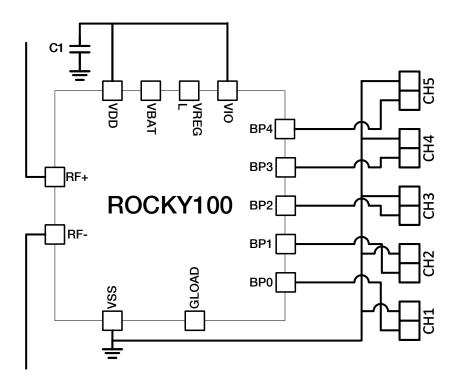
The ROCKY100 IC includes the RF frontend for UHF RFID power harvesting and communication, a power supply module to generate the required voltage levels, and an EPC C1G2/ISO18000-6C digital processor including a GPIO module. The GPIO module can be controlled via EPC C1G2 standard memory access commands.
