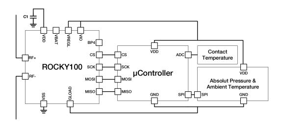
The ROCKY100 IC includes the RF frontend for UHF RFID power harvesting and communication, a power supply module to generate the required voltage levels, and an EPC C1G2/ISO18000-6C digital processor including a SPI bridge. The SPI bridge can be controlled via EPC C1G2 standard memory access commands.
