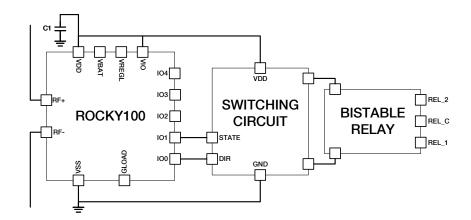
The ROCKY100 IC includes the RF frontend for UHF RFID power harvesting and communication, a power supply module to generate the required voltage levels, and an EPC C1G2/ISO18000-6C digital processor including a PWM module.
