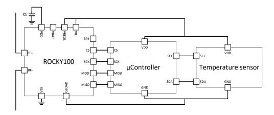
The ROCKY100 IC includes the RF frontend for UHF RFID power harvesting and communication, a power supply module to generate the required voltage levels, and an EPC C1G2/ISO18000-6C digital processor including a SPI bridge. The SPI bridge can be controlled via EPC C1G2 standard memory access commands.
